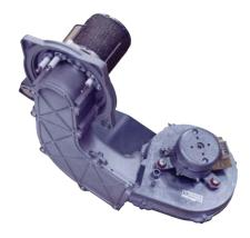
High efficiency, low restriction cylindrical shaped premix mesh burner and negative pressure gas valve allows a 5 to 1 boiler capacity turndown. DOE rated efficiency of 93% AFUE. Easy to access for scheduled maintenance.
