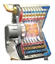
Patented 316L stainless steel full flow heat exchanger incorporates a tri-parallel flow design that yields high efficiency through even heat transfer and low water pressure drops. This radial flow heat exchanger is manufactured using robotic laser welding techniques for precision construction. "H" stamp ASME code certified.
